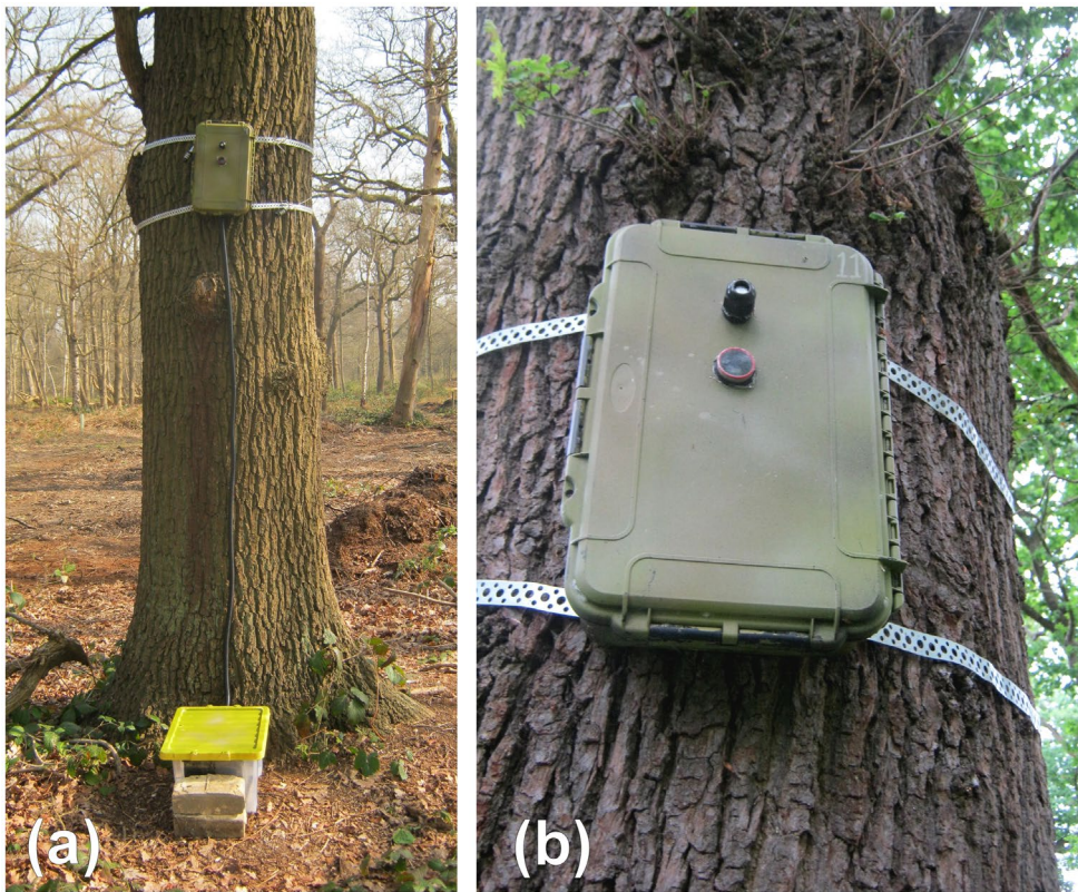
Figure 2. Examples of AURITA deployment configurations: (a) connected to a 12 V car battery in private locations (b) self-contained using USB power banks in public areas (Author's own).
